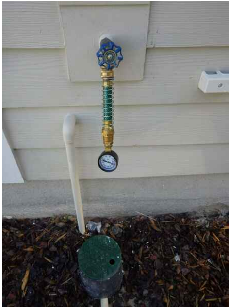
Water pressure measured 50 pounds per square inch
